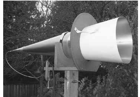
Here is a completed 144 MHz launcher, mounted to a wooden frame for testing.
