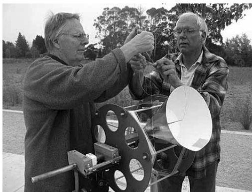
Completed 144 MHz launcher mounted on a "holder." The no. 24 SWTL conductor extends from the center of the horn and can be seen as a faint line in this photograph.
